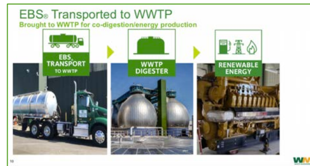
EBS transported to a wastewater treatment digester where it is converted to energy
