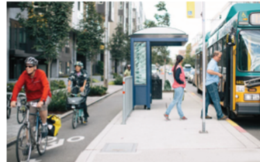
This roadway configuration, incorporating a protected bike lane and a raised bus stop, could be achieved by implementing a Road Diet
